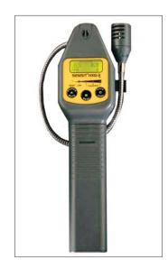
\* SENSIT® HXG-3 instruments are approved UL913, For Class 1, Division 1, Groups C, D, T3 hazardous locations when used with Duracell MN1400BK batteries or equivalent alkaline batteries.
