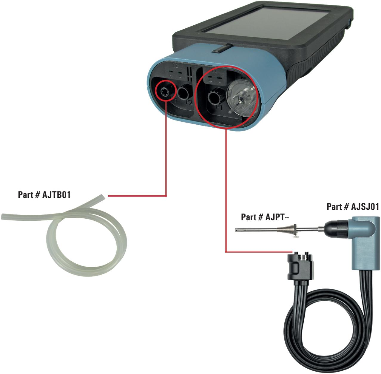
7.3 Connection of the instrument differential pressure measurement kit
