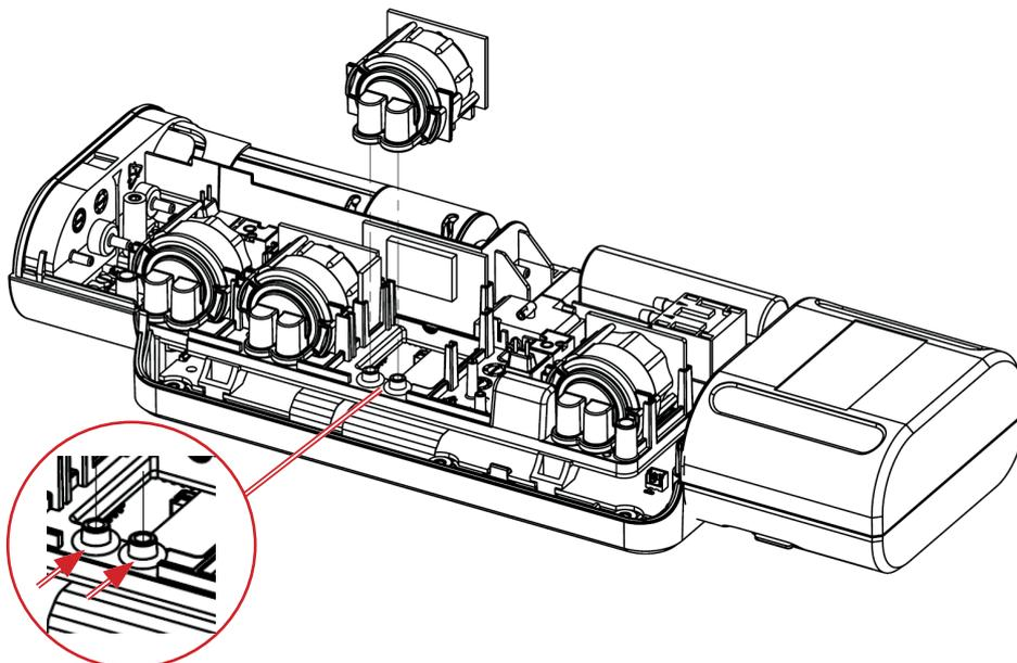
**When the sensor is removed, it is possible that two O-rings of the sensor itself remain stuck in the joints of the instrument (see the example in the picture below); it is necessary to remove them.**
