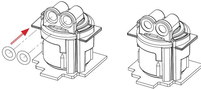
**The new sensors are provided with two O-rings; be sure that these O-rings are well inserted inside the special groove of the sensor (see the example in the picture below).**
