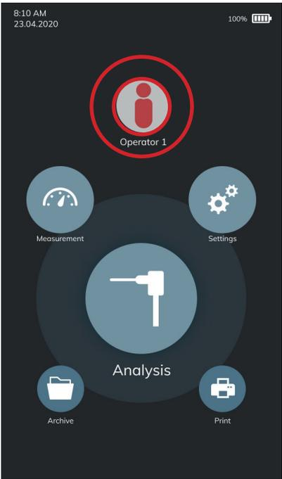
Press on the operator icon in order to select the operator name that will be printed on the instrument; the selected operator is highlighted in yellow.
