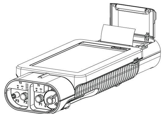
4. Close the entire printer cover assembly, applying a slight pressure on it in order to hook it to the instrument.
