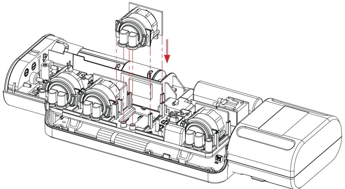
**Insert the new sensor into the rails and push down until fully seated.**
