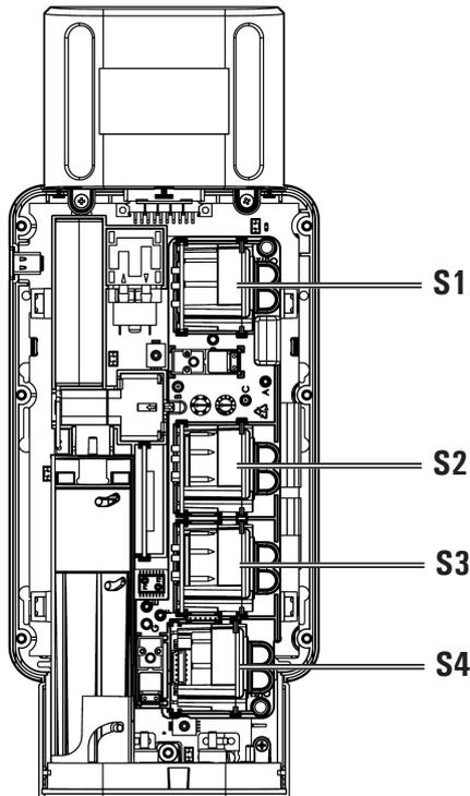
3. Once the position of the sensor to be replaced is located, pull upward the sensor.
