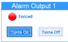
Fig. 46 – Alarm 1 output with forcing in on state
