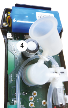
New sensor connected to electronic board
