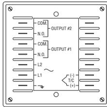
*Figure 3. Wiring Connections*
