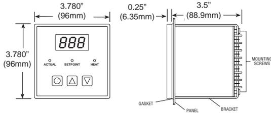
Before installing OTC25, ensure gasket seats evenly around edges of unit and that there are no breaks or tears in the gasket.
