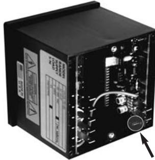
*Figure 6. Location of Calibration Jumper.*
