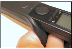
All operating elements and connections are still accessible if the protection boot is used.
