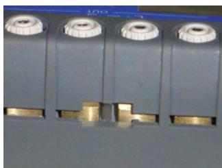
Connect your probes by simply pushing on the terminal top and insert wires of up to 3 mm or 10 AWG diameter and compensated thermocouple connectors. Wires are held tight between two brass plates ensuring thermal stability and a very good cold junction compensation for thermocouples. This system also enables 4 mm banana plugs and security connectors to be connected on the terminal top.
