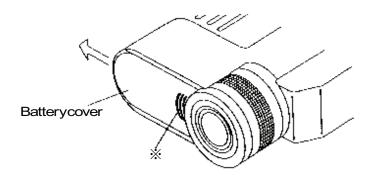
Removing the inside cover Remove the inside cover by turning the cover fixing screw in the arrow direction by using a coin.
