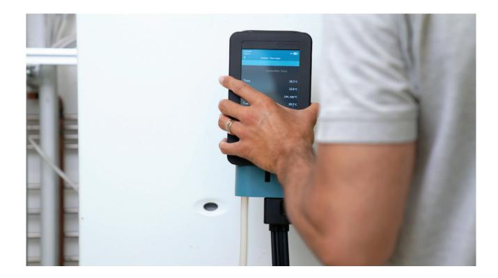
When performing a combustion analysis of the various combustion parameters, the user may often need also a pressure manometer, in order to simultaneously check and/or adjust gas pressures of the equipment. Thanks to the possibility of measuring combustion parameters and gas pressures at the same time, the newly developed Novo drastically reduces service time and limits the need to use different devices.
